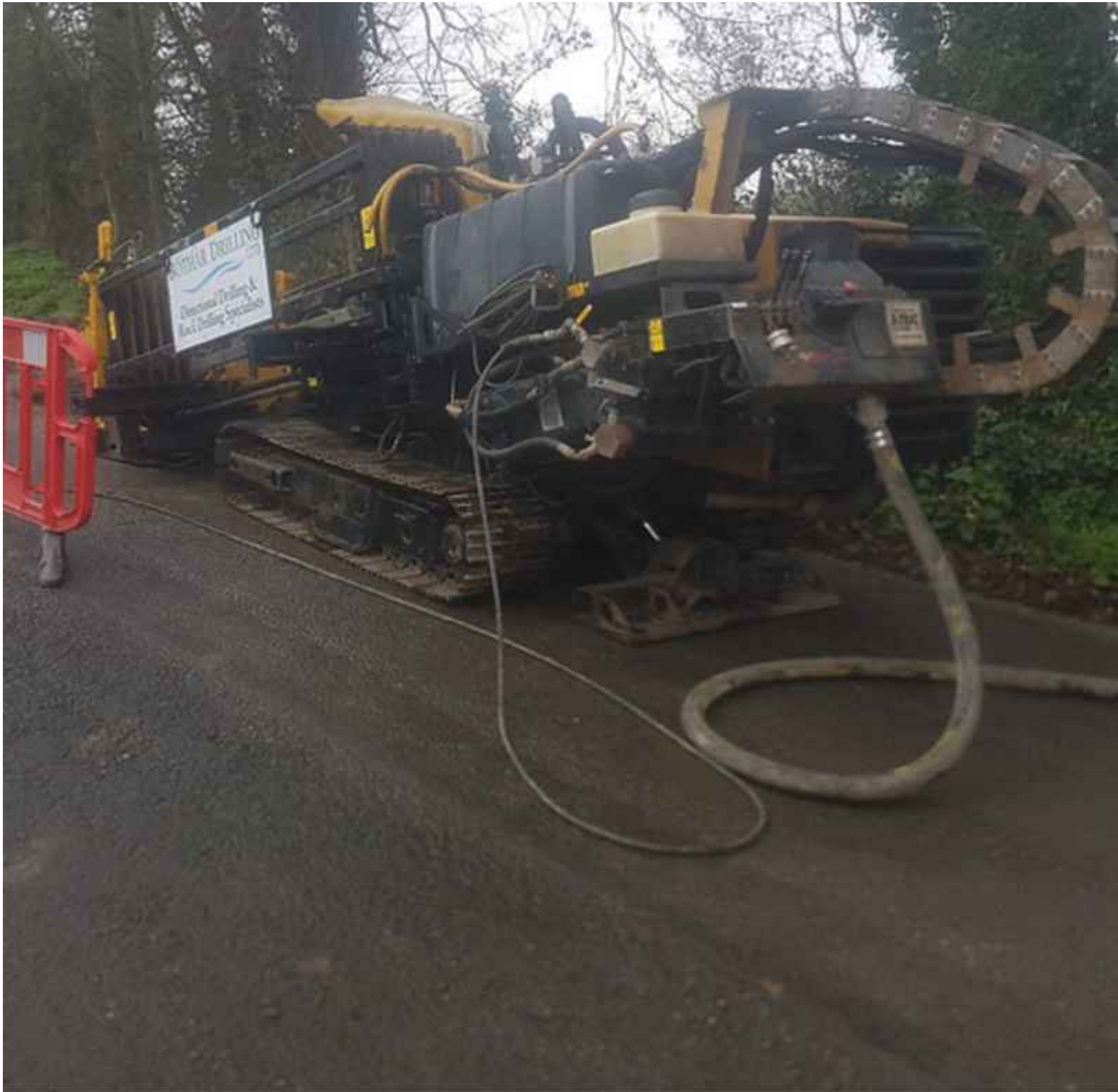
TYPICAL HDD DRILLING RIG
